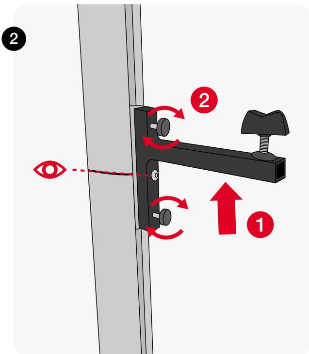
1. Position the arm so that the bolt aligns with the join of the two Twist extrusions.
