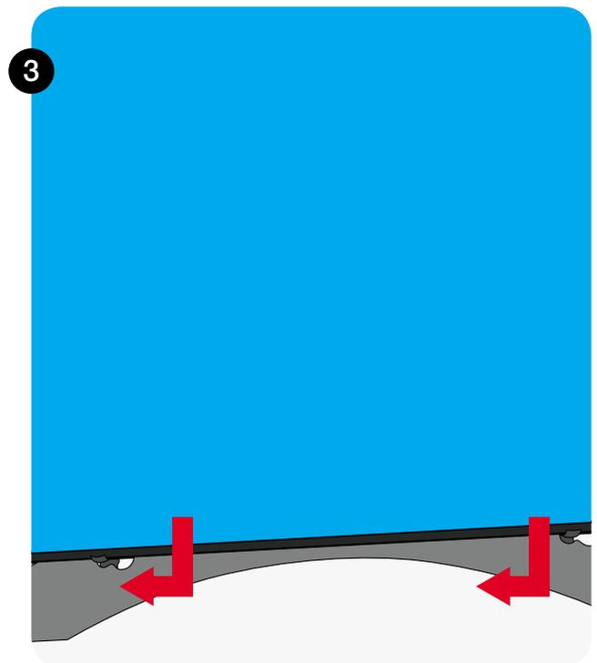
Pull down graphic and attach to the TWIST base.
