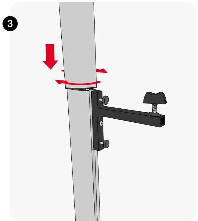
Attach top Twist extrusion.
